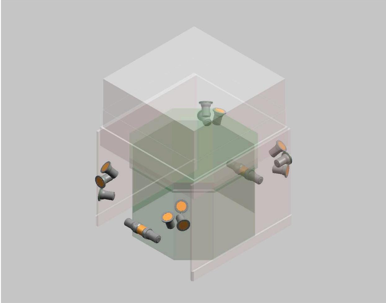
**Figure 3-2:** Placement of GBM Detectors on GLAST
